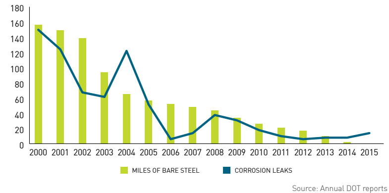
BARE STEEL PIPE REPLACEMENT COMPLETED IN 2015
