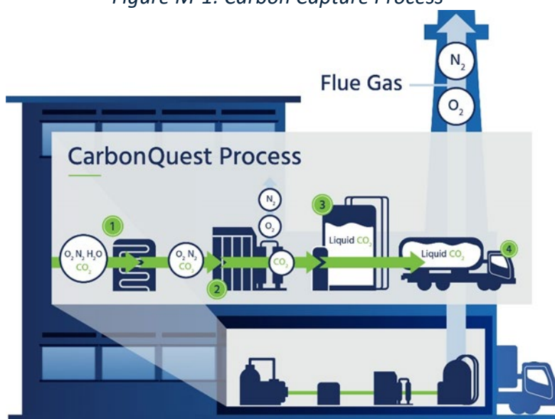
Figure M-1: Carbon Capture Process 25
